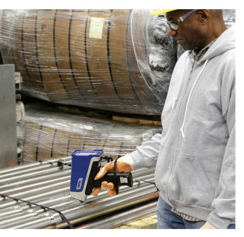
As the price of recycled metals fluctuates, identifying alloy grades quickly and easily is essential for profitability. Vanta™ handheld XRF analyzers for scrap sorting provide reliable identification in seconds for most alloys and pure metals.
